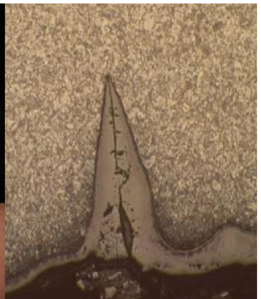
Cracking in a P91 tube-to-header weld
