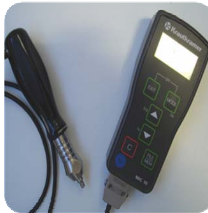
On-site hardness testing
